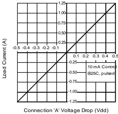
Figure 3. Linearity Characteristics
