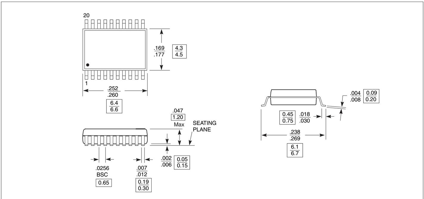
**Packaging Mechanical: 20-Pin SOIC(S)**
