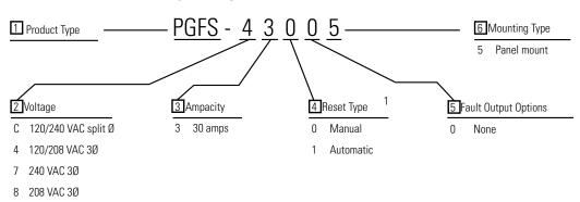
\*Note: 1. Manual configuration should be specified if automatic power-up, after power restoration of circuit power, could create an unsafe condition.
